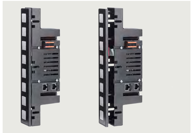
SIMATIC HMI KP8 PN LX, 8 short-stroke keys, long, 1–6 mm sheet thickness, PN interfaces, black neutral design, 8 configurable DI/DQ pins
